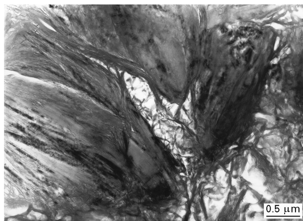
Figure 5 TEM micrograph of an Op region in the KOH-activated neat WPC paste. Op C-S-H not admixed with \text{Ca}(\text{OH})_2 is present in the centre and lower right of the micrograph.
